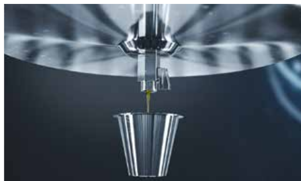
Liquid grease and impurities separated by TurboSwing® are removed with the opening of the tap.
