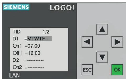
Exit the program menu by pressing Esc until, time and date appears on the screen, then press arrow ▲.
