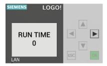
UV lamps have a lifespan of 8 000 h, then they should be replaced. The system will indicate when the run time of 8 000 h has been reached.
