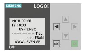
To stop the UV-purification manual press ( Esc + **◄** )
