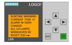
When the burning time of the UV lamps has reached 7 500 h an alarm is given that it is soon time to replace all UV lamps. Reset the alarm by pressing ESC + ▶
