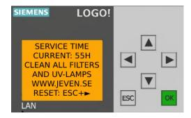
Reset alarm by pressing ESC+ ▶
