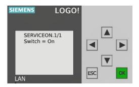
Adjust the cleaning interval if necessary. Default time is set to 55h (On =+00055).
