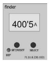
Window 3: Here you choose if you want to measure under or overcurrent, the system should me asure undercurrent and may not change! Press the "SET / RESET" button to proceed.
