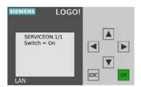
Adjust the cleaning interval if necessary. Default time is set to 10h (On =+00010).
