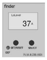
To check the current alarm limit and the ability to adjust it, you need to enter the Finder 71.51 programming view. Accessing the programming view is achieved by holding down the "Set/Reset" and "Select" buttons at the same time for 3 seconds.
