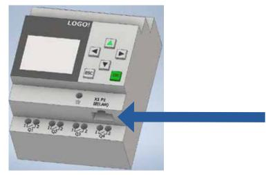
Connect the other side of Ethernet cable to the superior system, see example below:
