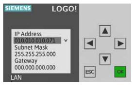
Press OK to start changing the IP address, use the arrow keys to change the numbers and move sideways. When the correct IP address is set, press OK.
