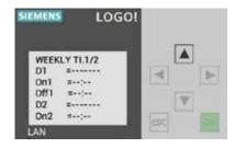
Exit the program menu by pressing Esc until, time and date appear on screen, then press arrow ▲.
