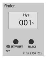
Window 6: (T1) Here you program a delay of outgoing alarm when it has detected a current loss, Finder 71.51 is programmed with a delay of 10 seconds. This value should not be changed. Press the "SET/RESET" button to proceed.
