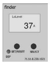
Window 5: Here is the value of the preprogrammed hysteresis value, this must not be changed! Press the "SET / RESET" button to proceed.
