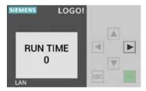
UV lamps have a lifespan of 8 000 h, then they should be replaced. The system will indicate when the run time of 8 000 h has been reached.
