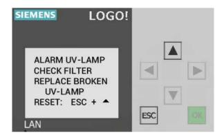
Refit the grease collector and reset the alarm by pressing ESC +  $\triangle$ .
