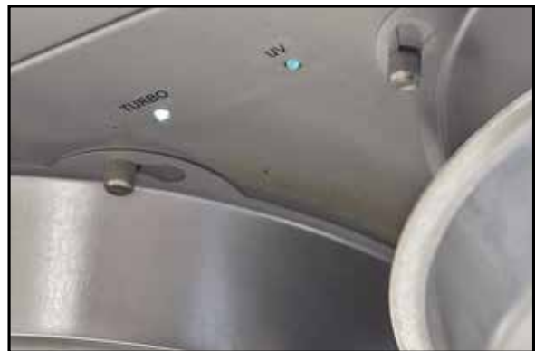
4 Make sure that the indicators for Turbo-filter and any UV light purification is lit.
