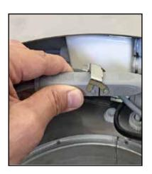
10 Connect motor with the quick coupling.
