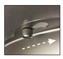
12 Reassemble the collection tub by lifting it in place and turning it clockwise. Tighten the screws.
