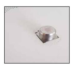
11 Refit the separation disc in the center of the motor shaft so that the square guide fits against the hole in the disc. Tighten the large nut carefully.
