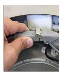
5 Disconnect motor with the quick coupling.
