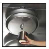
2 Open the valve on the filter. Empty the contents into a suitable container. Close the valve.
