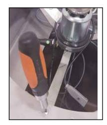
6 Remove the motor brackets by loosening three screws in the filter housing.
